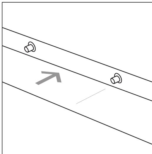
Verify that each panel's pins align correctly.
