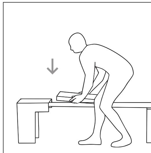
Slide panels into place, ensuring to align pins and holes.
