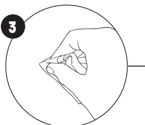
Using a microfibre cloth, wipe away any excess paint while ensuring the damaged area is fully covered.
