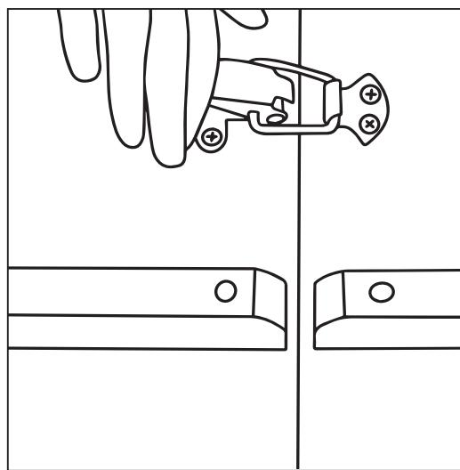
Secure panels using clips on the underside of the bench.
